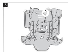
Insert the grommet (D) into the appropriate seat on the Acerbis skid plate (A).
