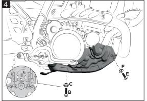
Position the skid plate (A) on the motorbike and fix it through the screw (B) and the bushing (C), the screws (E) and the bushings (F) on both sides.
